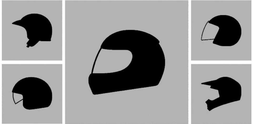
Different helmet makes, models and styles provide different head coverage and, as a result, the injury mitigation varies depending on the point of impact and the coverage area of the helmet.
